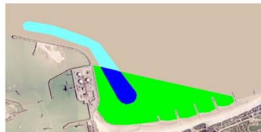
Figure 29. Qualitative representation of the sedimentation patterns in the Bay of Heist.
